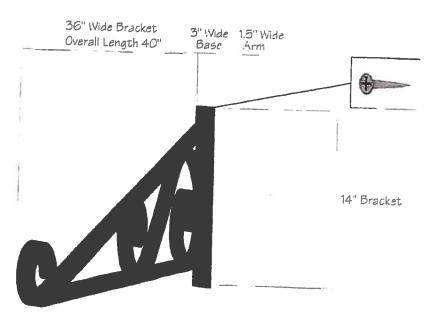
Lead shields with lag bolts, 3'' length, 3/8'' diameter, 4 total. Guy wire preferred if allowed,  $3'' \times 3/8''$  bolts with lead shield, 1/16'' coated stranded cable.
